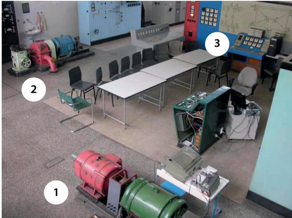
Figure 1. Miniature power system (1—thermal turbine; 2—hydro turbine; 3—transmission network).
