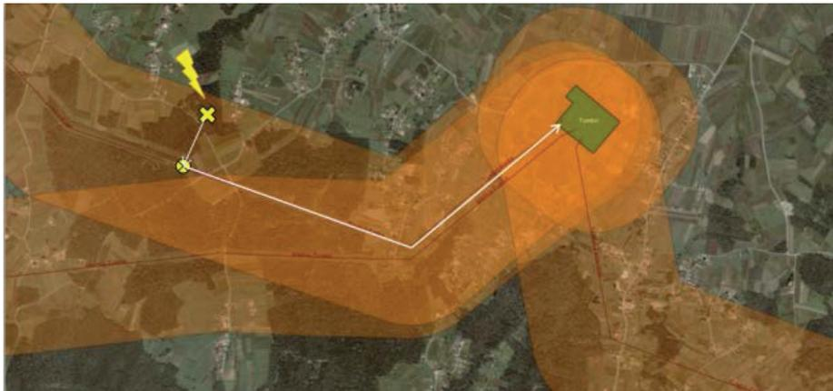
Figure 2. Spatial correlation of lightning stroke with overhead line alarm zones
