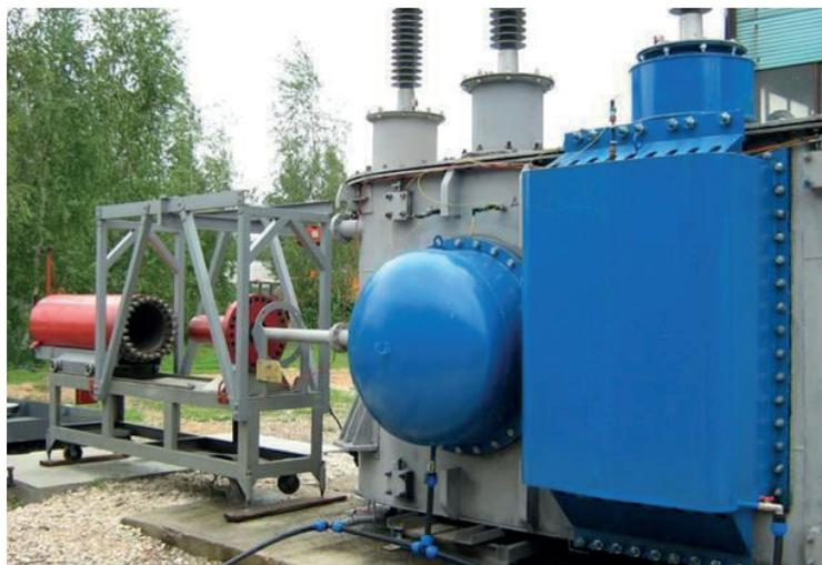
Figure 7 – Autotransformer with DPS before tests
