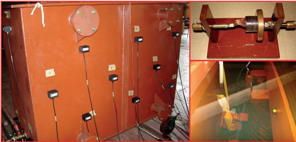
**Figure 2. Sensor placement (left), PD source (right up) and its placement in the tank (right down).**
