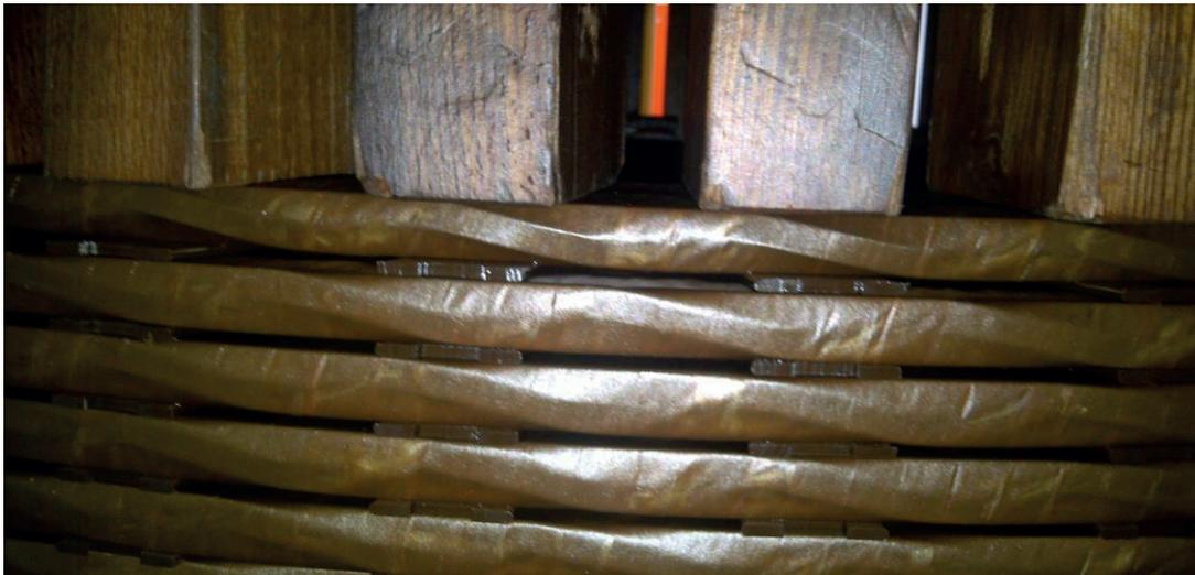
**Figure 12 – Model 3 under the influence of the 309% of the critical tilting pressing force according to IEC**
