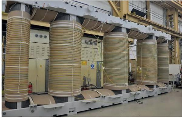
Figure 1 - Custom-made temporary windings during measurements
