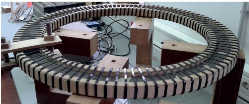
**Figure 7 – Magnetic steel ring used for experiment**
