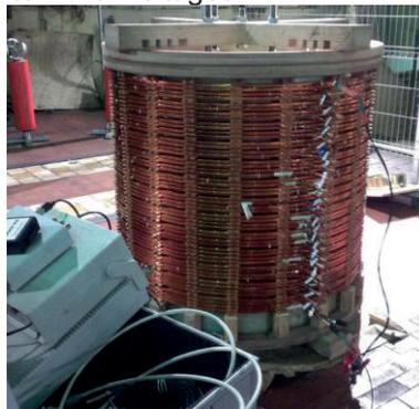
Figure 3 – Model of continuous disc-type winding
