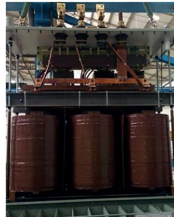
**Figure 5 – RDT after short circuit test**
