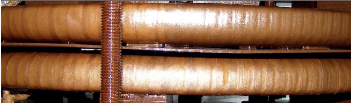
Figure 5 - Barrier distortion (the most prominent photo)
